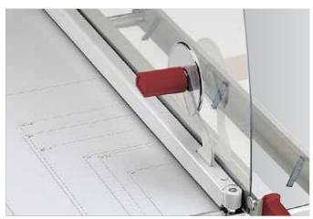
**SOLID MANUAL CLAMP** With this solid manual clamping device a variable clamp pressure can be applied depending on the material to be cut.
