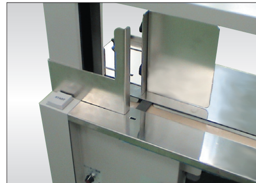
Auxiliary guide to bundle tags, labels, small packages and etc. easily.
